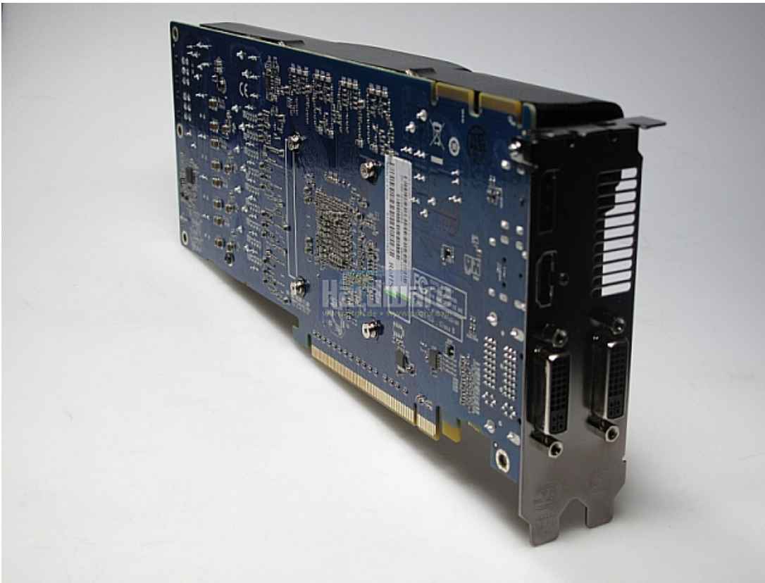
PCB view on one of the most successful GPU computing video cards, the Radeon HD 5870. Source: PC Games Hardware
